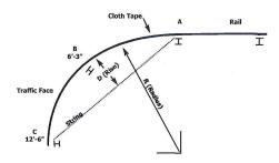
STEP 1: Starting at the last post in the straight run (point A), lay cloth tape along the path that the curved guide rail will follow.
