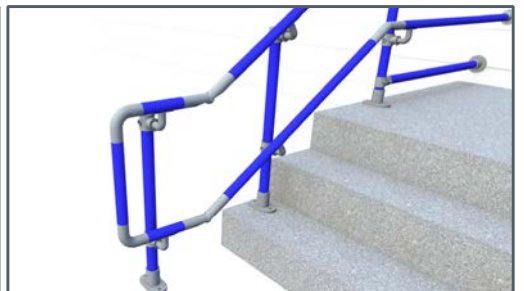
F) Extensions: Stairs: Railing should extend the width of one stair tread and then level out for 12". Ramps: Railing should extend parallel to walking surface 12" past the top and bottom of the ramp.
